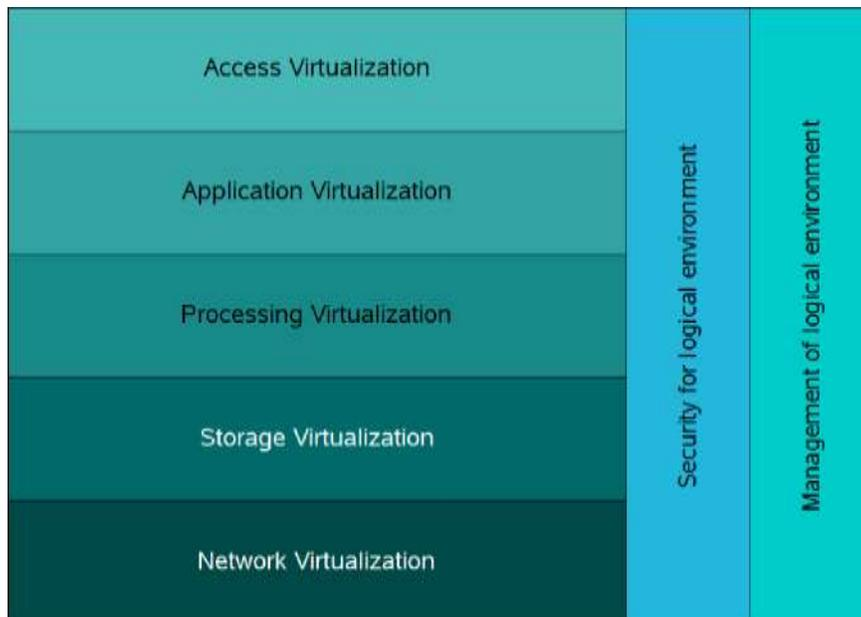
Processing virtualization hides the physical hardware configuration and makes it possible, on the one hand, to present a single system as if it were many or, on the other hand, to present many systems as if it were a single resource. Tools such as Intel® Virtualization Technology (Intel® VT) really help with the tasks found in this layer.
